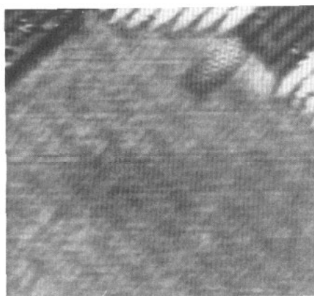
Figure 2. An enlarged section from figure 1, showing the (1 \times 1) structure. The contrast has been enhanced using a differential smoothing routine, but this has also reduced the magnitude, and hence visibility, of the buckling.
